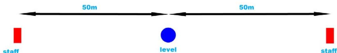
Finally, we planned to take staff readings with the level set up close to one staff and repeat with the level set up close to the second staff. These measurements would be used in conjunction with the dataset taken by the level at the mid-point to estimate of the systematic error in the level.
